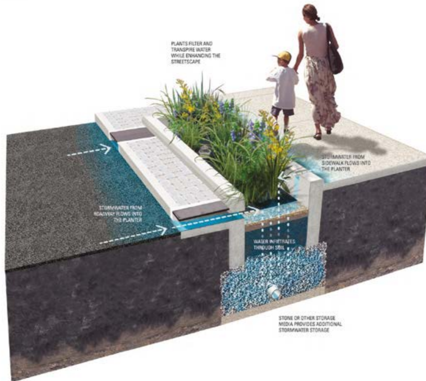
Figure 2.1: Three-Dimensional View of a Stormwater Planter
